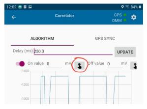
You will see a thick blue bar on the left side of the screen. Place your finger on the bar and drag to the On location.
