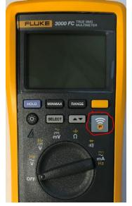
The Fluke screen will show 'Pair with', and the box next to 'App' will be solid. Press the Fluke 'select' button (second row on meter face)
