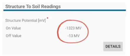
For Static or just ON readings you can select the Immediate button.
