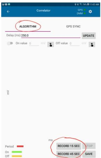
After the waveform capture is complete, we will select on and off values.
