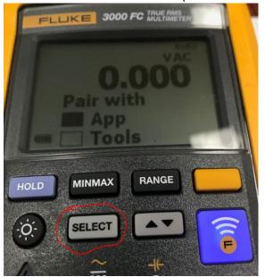
Now go to the tablet and select the 'Connect Fluke' button in the multimeter box.
